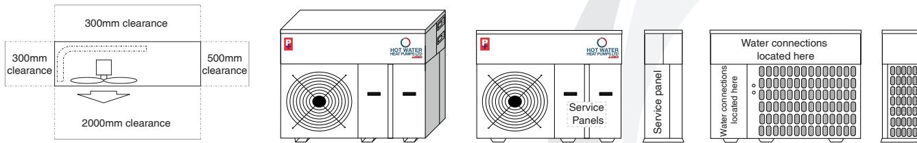
**Note:** 8G R32 Series heat pumps and chillers are not suitable for indoor/plant room installations without air quality monitoring and ventilation due to mild flammability.
